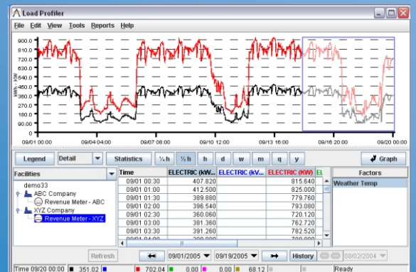
Query up to five days forward to receive a consumption and demand forecast based on the past five weeks.
